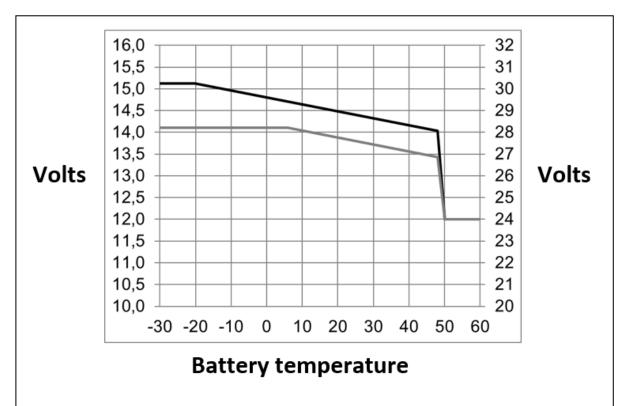
Default output voltages for Float and Absorption are at 25°C.
