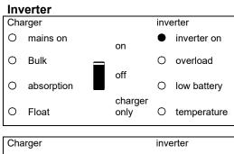
The inverter is on, and supplies power to the load.
